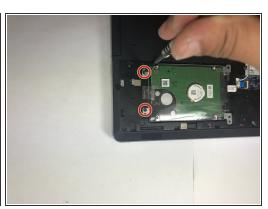
Remove each of the four (4) 2.5x8mm screws that anchor the hard drive using a Phillips #1 screwdriver.
