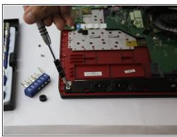
Remove the four screws, two on each speaker, with a PH1 screwdriver.
