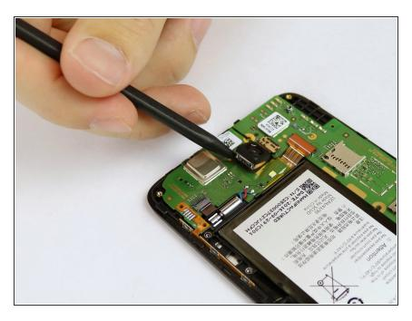
Pry out the camera with the pointy end of the spudger tool.
