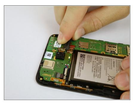
Use the flat end of the spudger tool to remove the connector.
