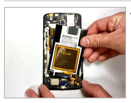
Remove the disconnected battery from the phone.
