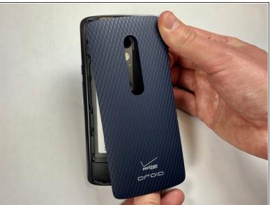
Wedge your thumb into the indent located on the bottom left corner of the back cover and pull up to remove the back cover.
