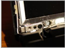
Remove the four screws (one in each corner) which attach the screen to the lid.
