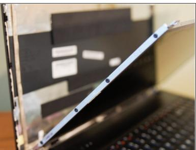
Remove the 8 screws (4 on each side) which attach the hinges to the screen
