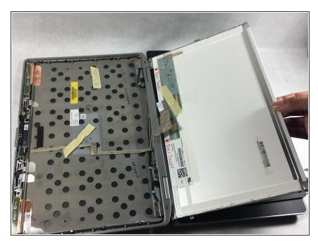
Lift the laptop screen and flip it over to lay it on top of the keyboard.
