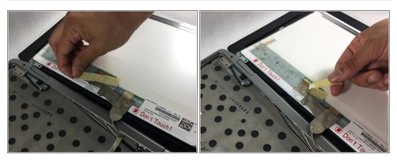
Remove the piece of tape from the back of the LCD cable.
