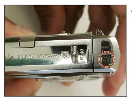
Remove the single Phillips #000 screw found next to the battery latch.
