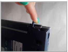
Pull the tab on the side of the optical drive till it pops out from the laptop
