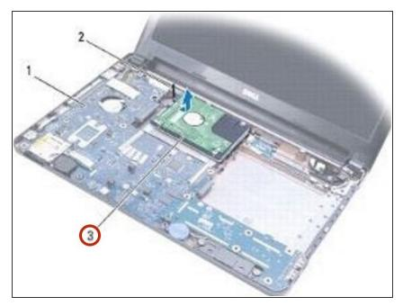
Place the hard drive in the computer base, then slide and connect the hard drive to the system board connector.
