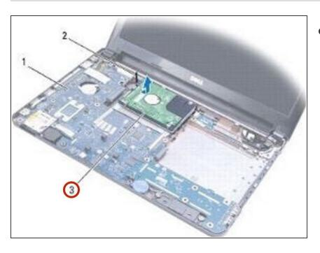
Lift the hard drive out of the computer base.
