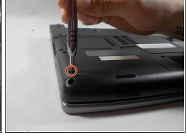
• Remove the two 6 mm Phillips #0 screws from the back of the hard drive cover.
