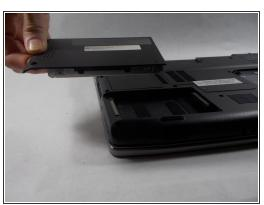
Press down firmly on the hard drive and pull leftwards.
