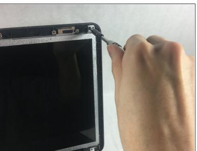
Remove four 4.0mm JIS #0 screws located at each corner of the monitor.
