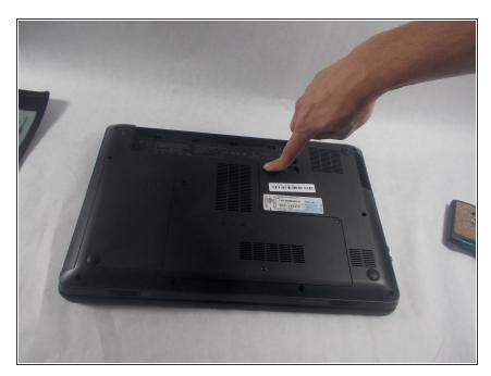
Slide pill shaped tab to the other side of the channel.
