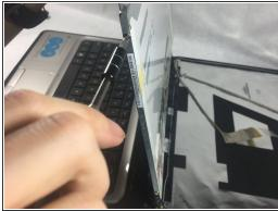
• Remove four 3.0mm JIS #0 screws, two on each side of the screen.
