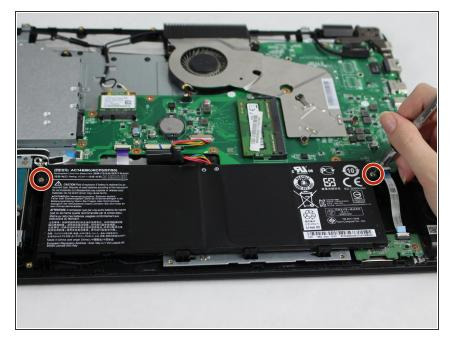
• Remove the two 5 mm screws located on either side of the battery.
