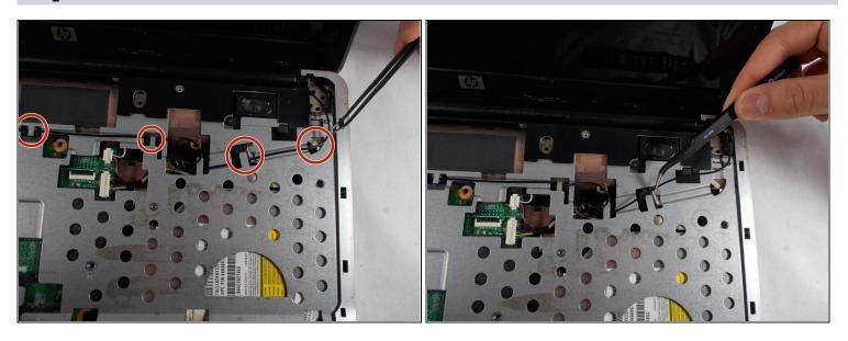
• At the top right of the laptop remove the black wire from under the metal tabs using the tweezers.
