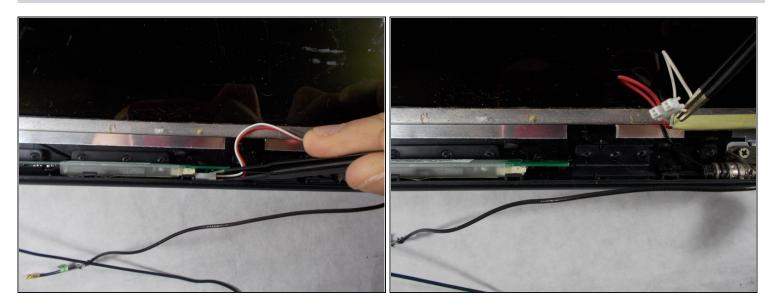
• Using the tweezers remove the red and white wire from the bottom of the screen.
