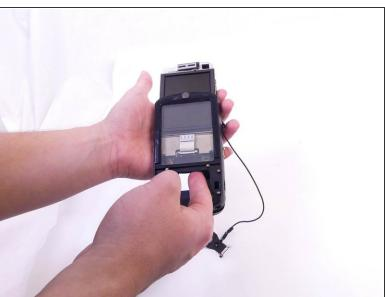
Using your finger, or spudger, push the motherboard out from the bottom.
