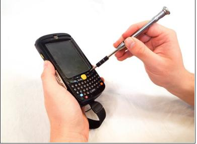
Remove the eight 4mm Phillips #00 screws from the keyboard cover.
