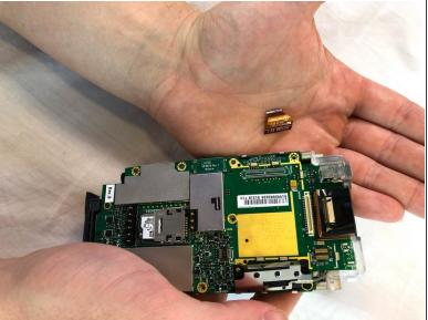
Remove the scanner ribbon cable by pulling straight up and out.
