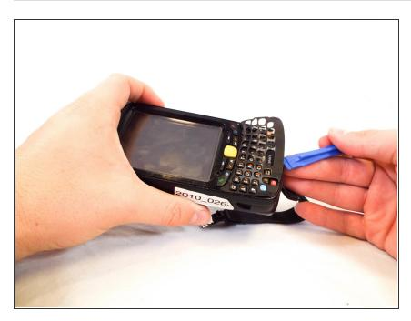
Use a plastic opening tool to remove the keyboard cover by prying up on its perimeter.
