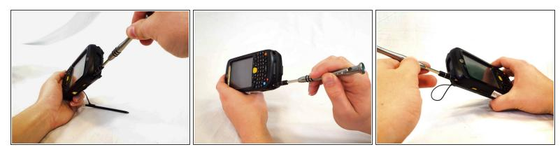
Remove the four 1cm Phillips #0 screws from the top and bottom of the phone.
