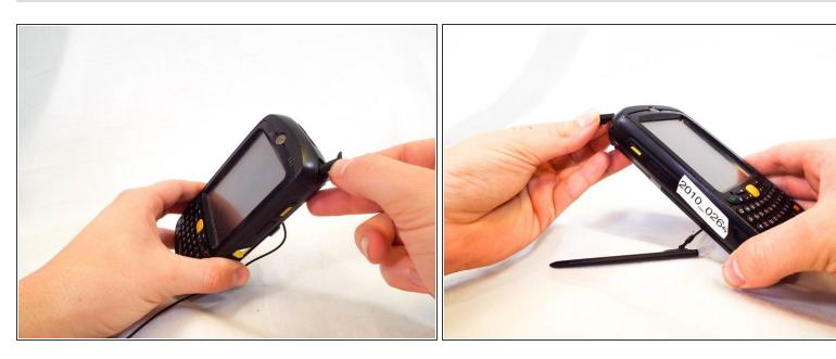
Remove the two rubber plugs on the top of the device by pushing them up and out of the phone.
