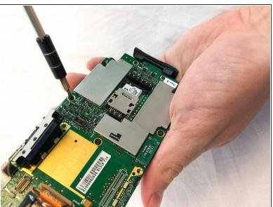
Remove the five 3mm Phillips #00 screws from the motherboard.
