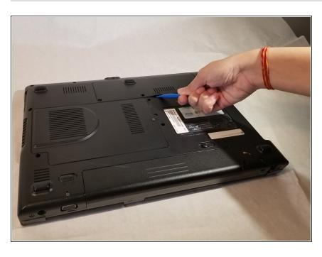
Using the plastic opening tool, pry open the plastic panel covering the hard drive.
