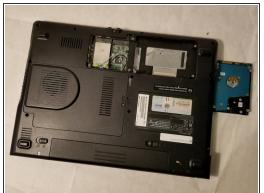
• Using your hands, carefully pull out the hard drive from its compartment.
