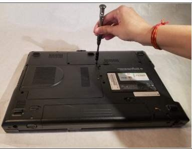
Using the Phillips #1 screwdriver, remove the three 6mm screws holding the hard drive panel in place.
