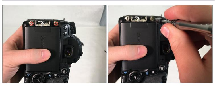
Remove two 4 mm Phillips #000 head screws that mount the LCD touchscreen to the hinge on the camera.
