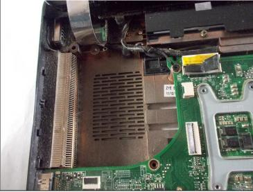
Pull up and remove the fan from the laptop.
