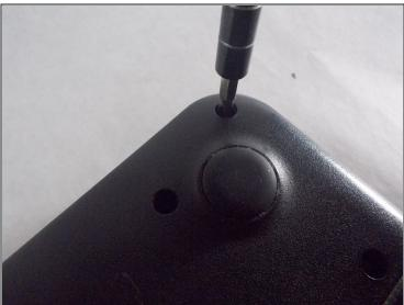
• Remove the 10 2.5x5 mm screws from the base of the laptop.
