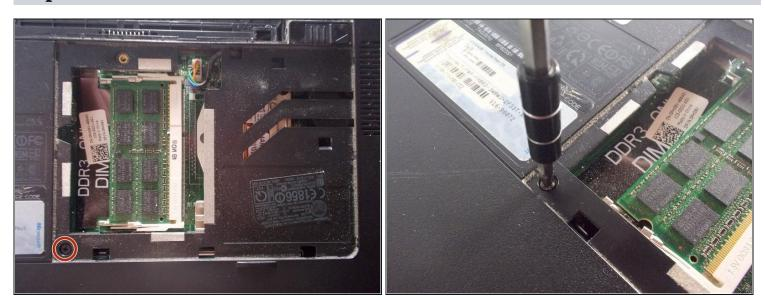
• Unscrew the 2.5x5 mm screw inside the RAM compartment.
