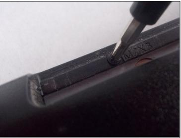
Unscrew the two 2x3 mm screws inside the disk drive compartment.
