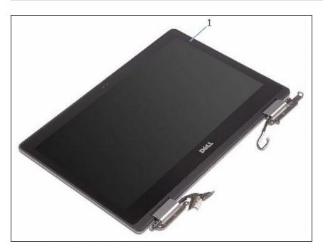
Place the display assembly face down on the palm-rest assembly.
