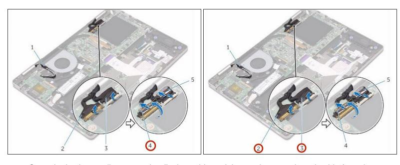
Open the latches to disconnect the display cable and the touch-screen board-cable from the system board.
