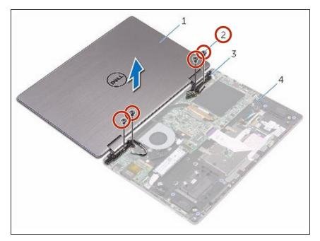
Replace the screws that secure the display assembly to the palm-rest assembly.
