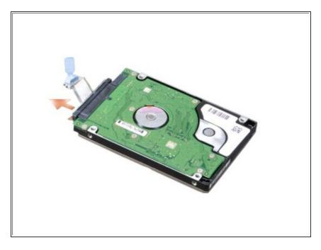
• Disconnect the hard drive cable from the connector on the hard drive..
