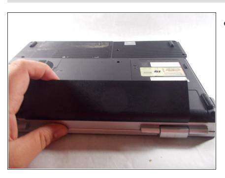
Remove the battery from its socket.
