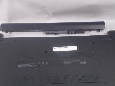
• Lift the battery from the middle and then pivot it outward to remove it from the computer.
