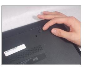
Firmly slide the release latch to unlock the battery and slide the battery release latch to release the battery.
