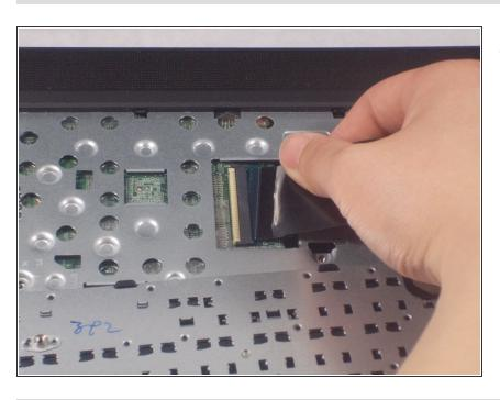
Disconnect the connected cable from the mainboard.
