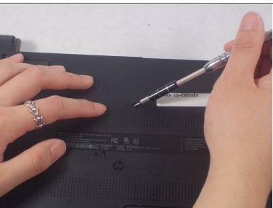
Remove the single 7 mm screw from the top middle of the laptop using a Phillips #0 screwdriver.
