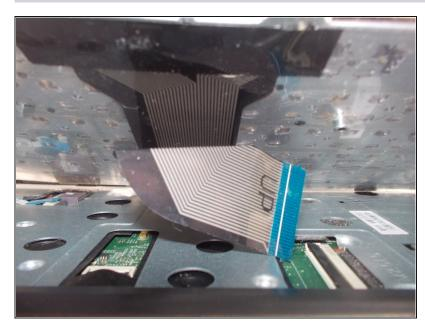
• Carefully disconnect the ribbon cable from the socket and pull apart.
