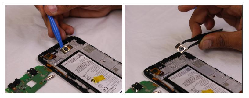
Use a plastic opening tool to pry up the camera.
