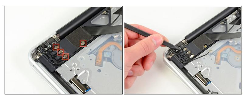
Use the tip of a spudger to pry the four antenna connectors up from their sockets on the AirPort/Bluetooth board.
