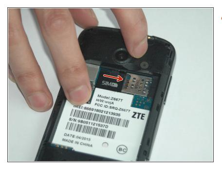
Press the small black tab and insert the micro SIM card with the metal contact facing downwards.
