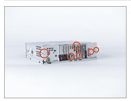
Remove the six 5mm Phillips-head screws with Philips #2 screwdriver.
