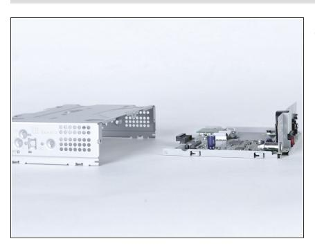
The metal casing is now fully removed.
