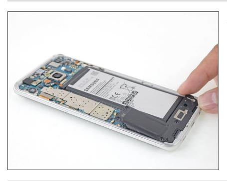
Lift and remove the loudspeaker from the phone.
