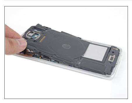
Lift and remove the wireless charging coil from the phone.
