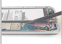
• Use the pointed end of a spudger to disconnect the red and white antenna cables.
