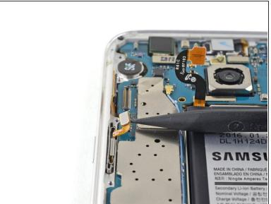
• Use the pointed end of a spudger to disconnect the power button cable.
