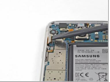
• Use the flat end of a spudger to disconnect the display cable.
