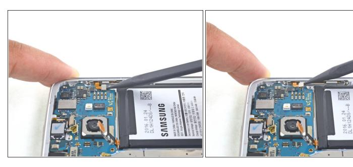
Use a pointed end of a spudger to disconnect the volume button cable.
