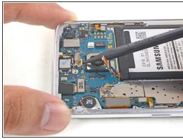
• Use the pointed end of a spudger to disconnect the front-facing sensory array cables.
