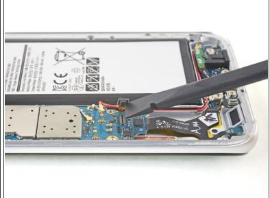
Use the flat end of a spudger to disconnect the home button connector.
