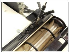
Remove the four 10 mm screws with a Torx T10 screwdriver.
