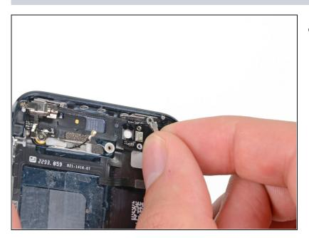
Remove the metal bracket between the rear facing flash and camera windows.
