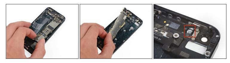
• Rotate the logic board assembly toward the battery side of the rear case.
