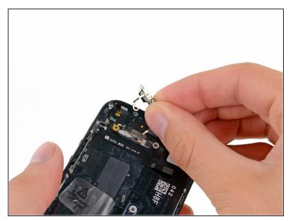
Remove the vibrator and vibrator bracket from the rear case.
