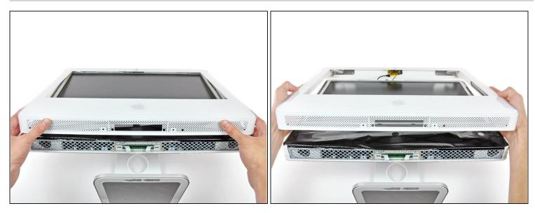
• Lift the front bezel off the rear case and rotate it away from the bottom edge of the iMac, minding the camera and microphone cables still attached to its upper edge.
