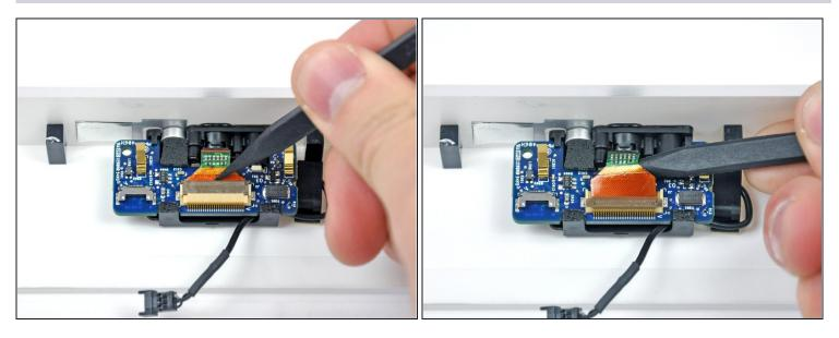
• Use the tip of a spudger to flip up the camera ribbon cable retaining flap.
