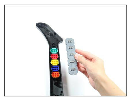
Using your fingers, remove the rubber pad to expose the colored keys.
