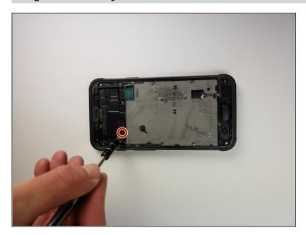
Use a Phillips #000 screwdriver to remove a single screw.
