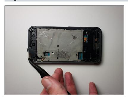
Use tweezers to take out the middle button and its connection to the motherboard.
