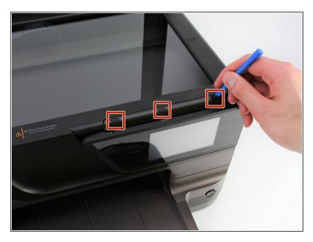
Wedge the plastic opening tool into each of the three plugs to pry them from the control panel hinge located above the control panel screen.
