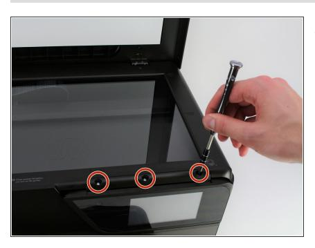
Remove the three 10mm-T10 Torx screws.
