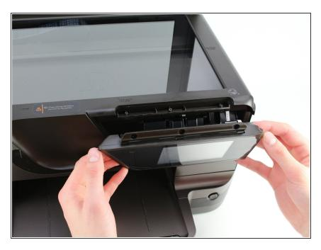
Disconnect the control panel from the hinge by gently lifting upward, then outward towards you.
