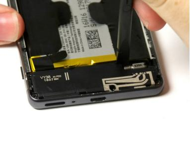
Push back the two retaining tabs on the top of the loudspeaker with the spudger.
