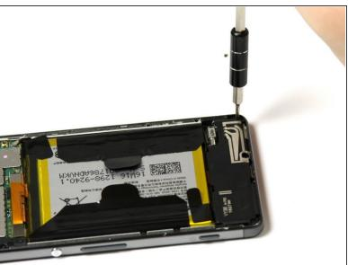
Remove the four 4mm screws holding the loudspeaker in place with a Phillips #00 screwdriver.
