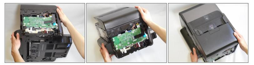
• Rotate the printer to its standard position.
