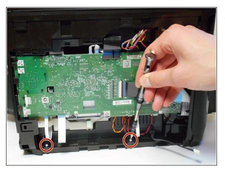
Remove the two 12mm-T10 Torx screws from the base of the power supply mount.
