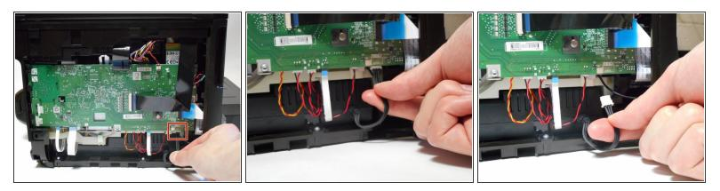
• Unplug the black wire with the white cap connecting the power supply to the motherboard.
