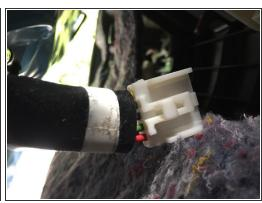
• There is one electrical connector for the door light that need to be removed in the panel. From the bottom of the door, with the panel opened up, I pressed in on the tab in the middle of the harness connector will release the harness and simultaneously then we need to pull the harness down, away and out of the mating connector
