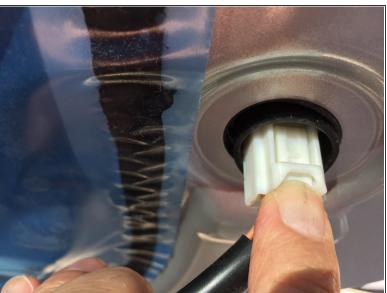
Remove the door lock actuator wiring harness by pressing the harness tab and simultaneously pulling it back and out of the connector housing.
