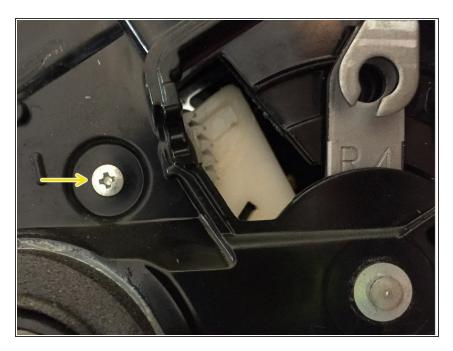
After removing the cable, remove the small screw located adjacent to the compartment. Set the screw aside for reassembly.
