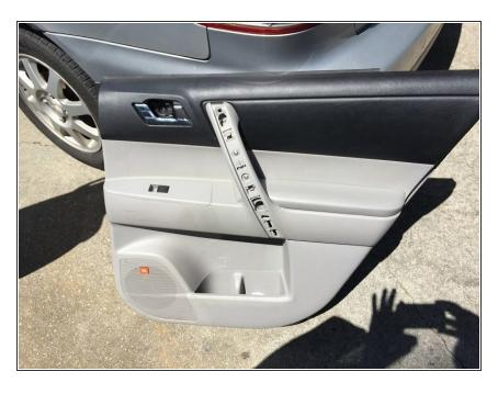
With the electrical connector released, work the top of the door panel out of the clips along the top at the window slot. This took me way
