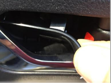
Remove the black plastic cover "plate" behind the door handle. I pulled open the door handle and used a metal spudger in the lower right corner to pop out this cover plate.
