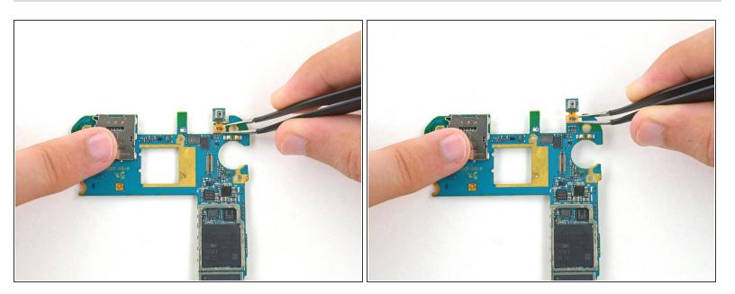
Remove the microphone from the motherboard.
