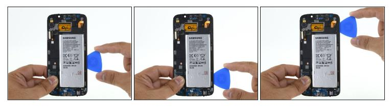
Slide the pick along the edge to cut through the adhesive.
