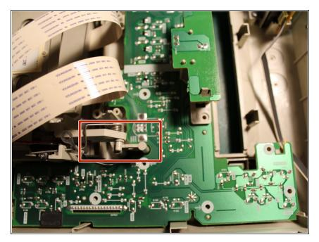
carefully lift up one side of the cassette deck and remove the pcb
