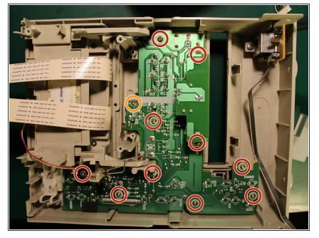
Remove the screws (you have to remove the casetdeck to access the orange screw)
