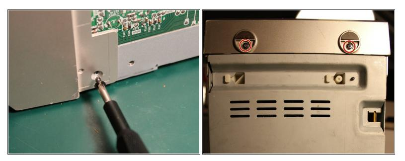
Remove the screws on both sides and on the bottom
