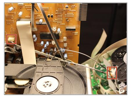
Remove the front and the rest of the cables
