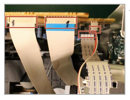
Remove the flex cables with easy access
