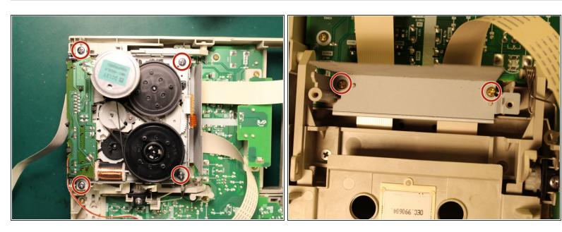
Remove the cassette deck (this is to access the screw beneath it)
