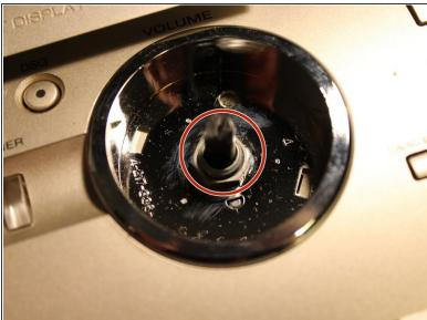
Remove the volume knob and the screw behind it
