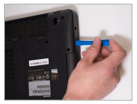
Insert a plastic opening tool in between the panel and the main assembly.
