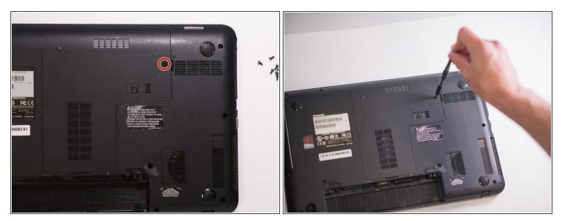
Remove the 7mm Phillips screw located on the easy access panel on the bottom of the laptop using a Phillips #1 screwdriver.
