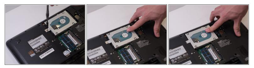
Remove the 3mm Phillips #1 screw holding the HDD in place, then slide the HDD towards the sticker.
