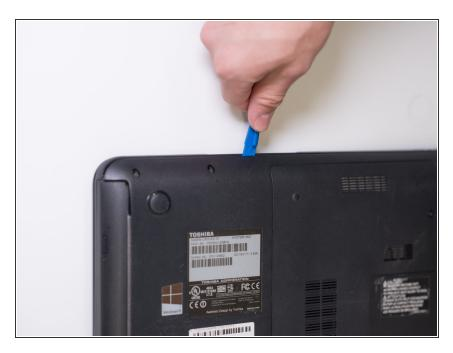
• Work your way around the laptop to remove the base plate.
