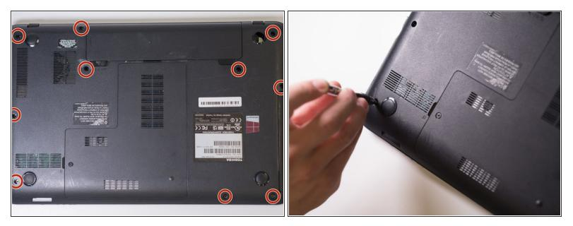
Remove the ten 7mm Phillips screws located on the bottom of the laptop using the Phillips #1 screwdriver.
