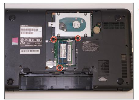
Remove the three 3.5mm Phillips #1 screws indicated in the picture.
