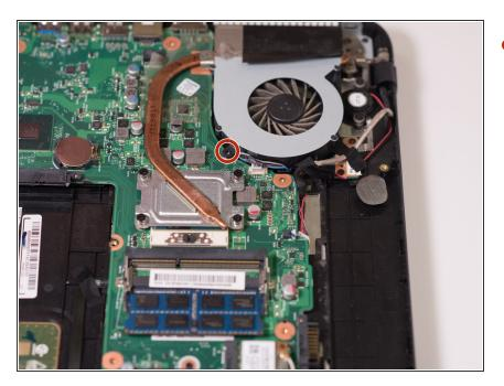
Remove the single 1.5mm Phillips #1 screw located next to the cooling fan.
