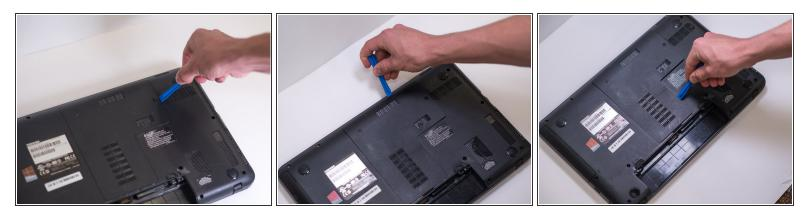
Insert a plastic opening tool and follow the edges to open the panel.
