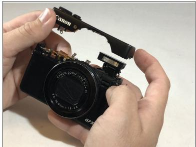
While using the plastic opening tool, gently pry the top plate off the camera.
