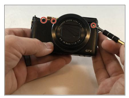
Take the Phillips #000 and remove the three 5 mm screws from the front plate.
