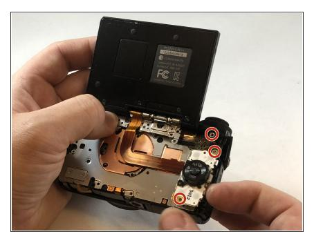
Remove the three 3 mm Phillips #000 screws around the dial.
