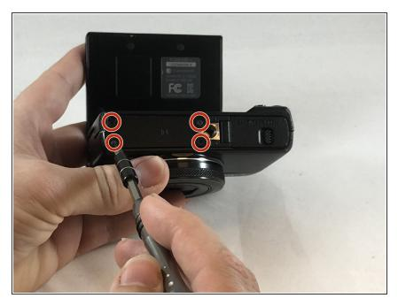
Remove the four 4 mm Phillips #000 screws from the plate on the bottom of the camera.
