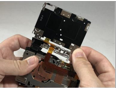
Using the black nylon spudger, gently lift the ribbon cable connected to the LCD screen housing until it comes out then remove the housing.
