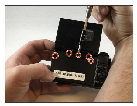
Remove the five 2mm Phillips #000 screws that are under the screen of the camera.
