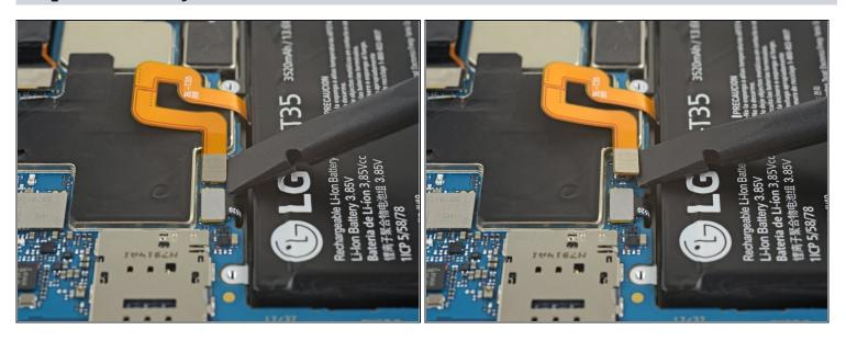
Use the flat end of a spudger to disconnect the battery connector.
