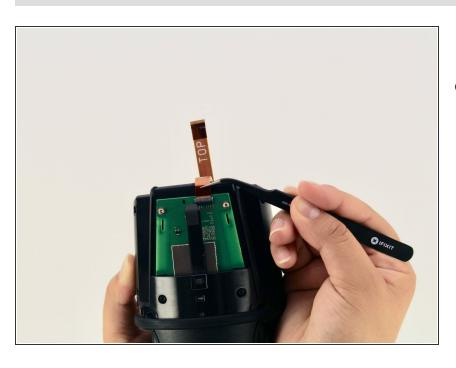
Carefully remove the interconnect cable using a pair of tweezers. To reassemble your device, follow these instructions in reverse order.
