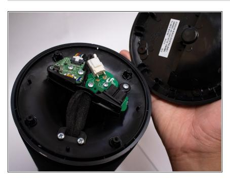
Remove the bottom shell from the speaker.
