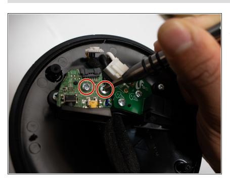
Remove the two 10mm long screws from the board utilizing the Phillips #1 screwdriver.
