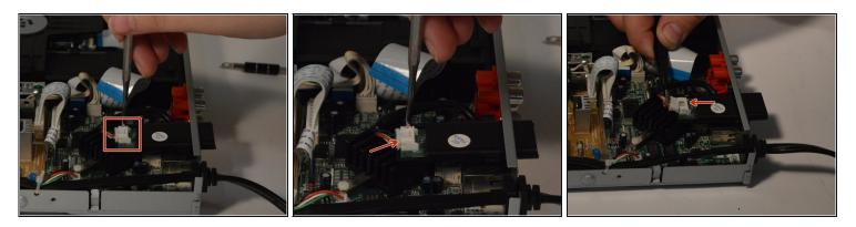
• Use the metal spudger to remove the white clip from the antenna by prying the clip away from the antenna.
