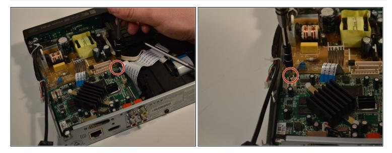
• Remove the two 5mm screws that connect the mother board to the device.
