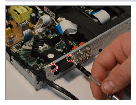
• Remove the two 7mm screws from both sides of the antenna.
