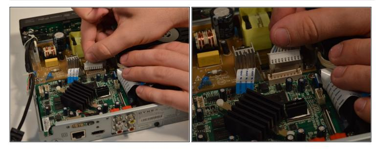
• Pull the larger white 9 pin power cord that connects the power board to the motherboard.
