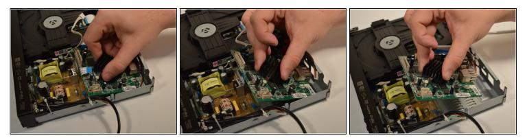
• Slide board up and out at a slight angle
