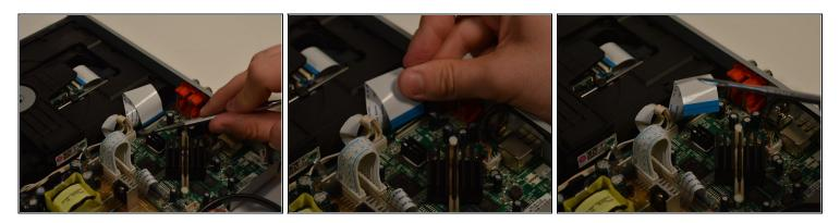
• Lift up and out to remove the large white plastic wiring strip. Lift lightly on the back clip holding it to loosen.
