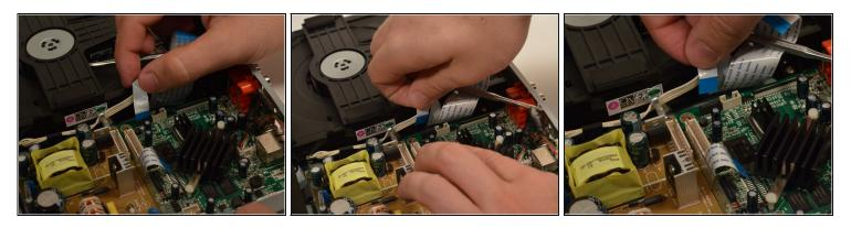
• Pull the second white 1cm wide tab between the motherboard and power supply board.
