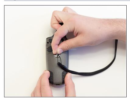
Lift and twist the battery cover release 90 degrees counterclockwise on the back of the device.
