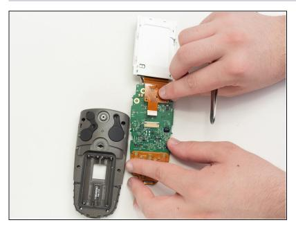
• Remove the screen ribbon connector and screen.
