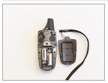
• Lift battery release up to remove battery cover.
