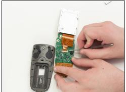
Use tweezers to pull the two white pins on the connector forward.
