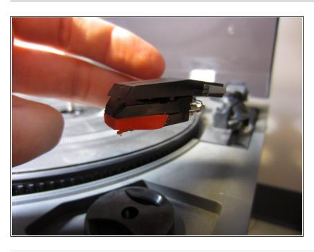
Insert a new stylus by pushing it back up where the old one was, or, if necessary, clean the old one and replace likewise.
