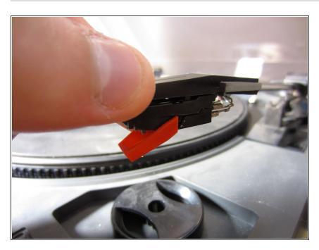
Press down on the front of the red stylus and pull forward to remove it from the arm.
