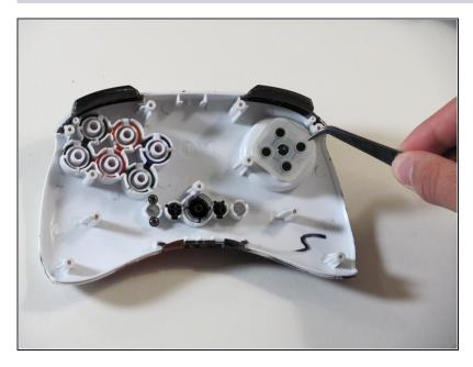
Use <u>tweezers</u> to remove the rubber part of the directional pad.
